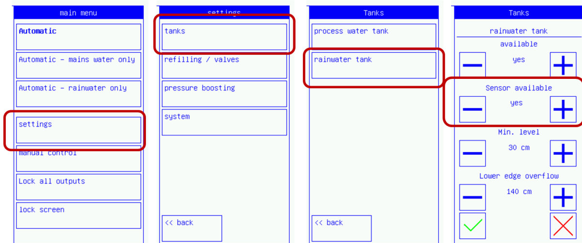
Figure 50: Activation of the sensor for the visualisation of the filling level
